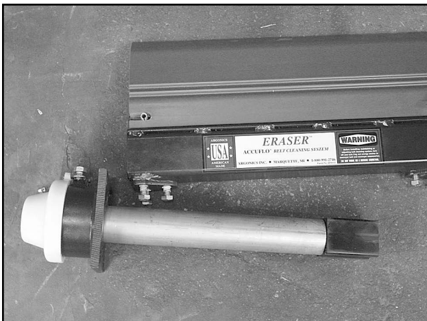
Using a ½" end wrench, loosen the three setscrews located on the bottom of each end of the mainframe. Remove the entire tension cartridge from the left side of the mainframe.
